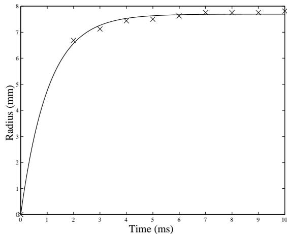
**Figure 9.** This plot shows the radius of a carbon cloud formed at 2000psig as a function of time.
