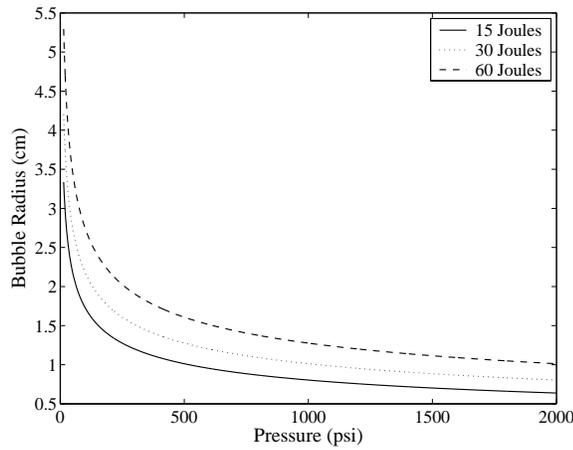
**Figure 1.** Plots of the maximum bubble radius versus pressure for three energy levels
