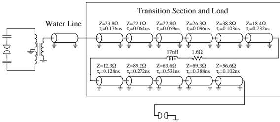
**Figure 6.** Transmission line model used to simulate the risetime of the circuit
