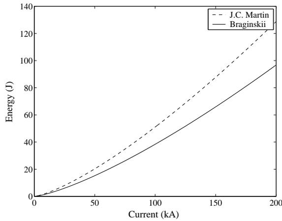
**Figure 3.** Comparison of the J. C. Martin energy loss approximation to the Braginskii loss method for a range of currents.
