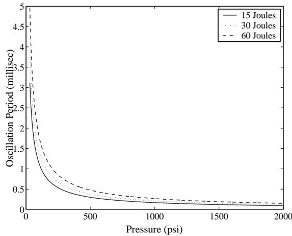
**Figure 2.** Plots of the oscillation period versus pressure for three energy levels
