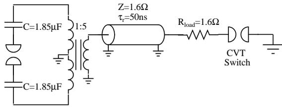
**Figure 5.** Single shot experimental test circuit for CVT switch
