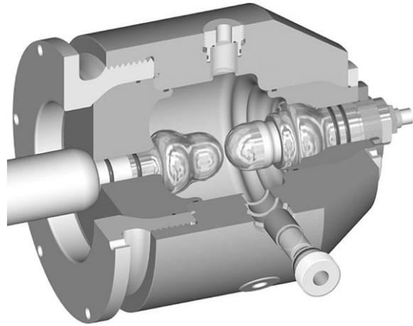
**Figure 4.** Cross section of the CVT switch with hemispherical electrodes, view ports, and oil ports.
