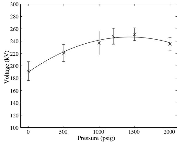
**Figure 8.** This plot shows the average breakdown voltage for a 0.2cm gap at various pressures with one standard deviation error bars.
