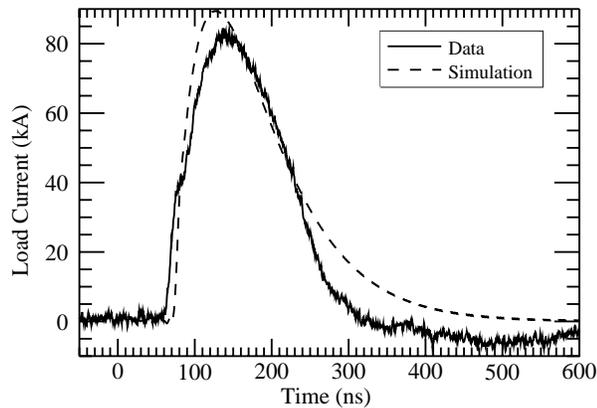
**Figure 6.** Comparison of a BERTHA simulation to Rogowski coil current measurements for a six cavity LTD shot at SNL.
