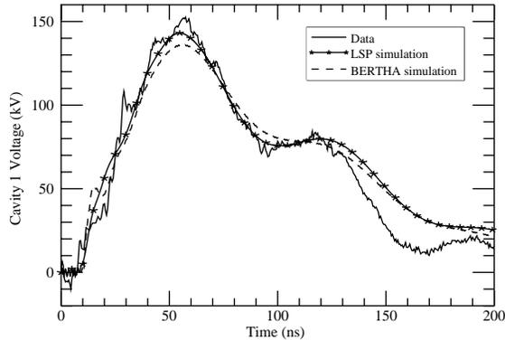
**Figure 3.** Comparison of simulations of the 1 MV LTD to Cavity 1 voltage measurements from experiments at HCEI.
