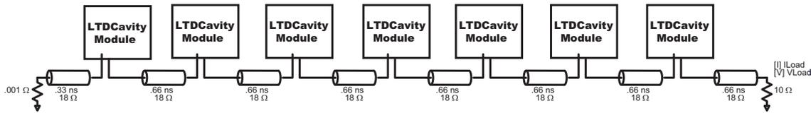
**Figure 2.** Diagram of the main BERTHA circuit file used to simulate the LTD. Each “LTD Cavity Module” block links to a circuit description of a single LTD cavity.
