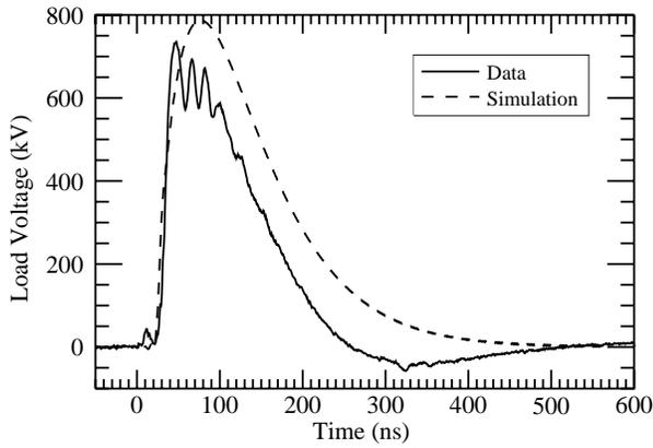
**Figure 5.** Comparison of a BERTHA simulation to the sum of cavity voltage measurements from experiments with six series LTD cavities.
