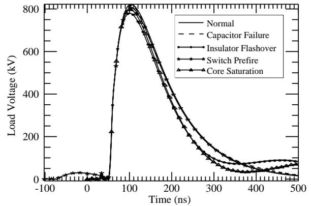
**Figure 7.** Comparison of simulated load voltages for various LTD fault modes. The peak load voltage is decreased by no more than 6% for any of the simulated faults.
