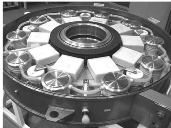
**Figure 1.** Photograph of the inside of a single cavity of the 1 MV LTD.
