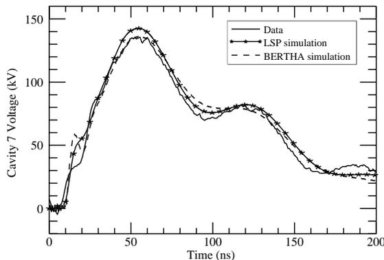
**Figure 4.** Comparison of simulations of the 1 MV LTD to Cavity 7 voltage data.
